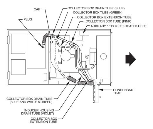
Fig. 11—Horizontal Right Tube Configuration
